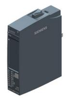
SIPLUS ET 200SP, digital input module, DI 16X DC 24V standard, -40...+70°C with conformal coating based on 6ES7131-6BH01-0BA0 . type 3 (IEC 61131), sink input, (PNP, P-reading), Packing unit: 1 Piece, passend für BU-Typ A0, Farbcode CC00, Modul-Diagnose input delay time 0,05..20ms, diagnostics wire break, diagnostics supply voltage
