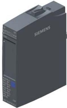
SIPLUS ET 200SP AI 8xRTD/TC 2-wire -40...+60 °C with conformal coating based on 6ES7134-6JF00-0CA1 . analog input module, AI 8xRTD/TC 2-wire high feature FITS to BU type A0, A1, color code CC00, channel diagnostics, 16-bit, +/-0.1%
