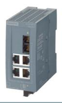
SCALANCE XB004-1LD unmanaged Industrial Ethernet Switch for 10/100 Mbit/s; for setting up small star and line topologies; LED diagnostics, IP20, 24 V AC/DC power supply, with 4x 10/100 Mbit/s twisted pair ports with RJ45 sockets; 1 x 100 Mbit/s single-mode glass fiber-optic cable port with SC socket; manual available as a download .
