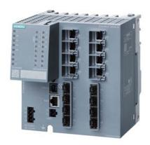
SCALANCE XM408-8C; managed modular IE switch; 8x 10/100/1000 Mbit/s RJ45; 8x 100/1000 Mbit/s SFP; contains 8 combo ports; in total 8 ports can be used; expandable to 24 ports electrical or optical; assembly: DIN rail/S7 mounting rail, PROFINET IO device; redundancy functions; office features (RSTP, VLAN, IGMP,...); C-plug in scope of delivery; Layer 3 with key plug available
