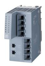
PE408PoE Port Extender for SCALANCE XM-400 managed modular IE switch; extension by 8x 10/100/1000 Mbit/s RJ45 with up to 8 ports PoE according to IEEE802.3AT; for PoE separate power supply required
