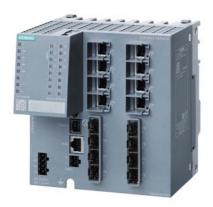
SCALANCE XM408-8C; managed modular IE switch; 8x 10/100/1000 Mbit/s RJ45; 8x 100/1000 Mbit/s SFP; contains 8 combo ports; in total 8 ports can be used; expandable to 24 ports electrical or optical; assembly: DIN rail/S7 mounting rail, PROFINET IO device; redundancy functions; office features (RSTP, VLAN, IGMP,...); C-plug in scope of delivery; Layer 3 integrated
