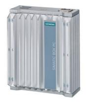
SIMATIC IPC127E; Atom E3940 (4C/4T), 4 GB RAM; Extended version; 3x Ethernet RJ45, 4x USB3.0; Windows 10 Enterprise LTSB 2016, 64 bit, MUI (en, de, fr, it, es); 64 GB SSD; without mounting accessories
