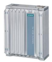
SIMATIC IPC127E; Atom E3930 (2C/2T), 2 GB RAM; Extended version 3x Ethernet RJ45, 4x USB3.0; without operating system; 64 GB SSD; without mounting accessories
