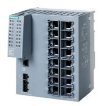
SCALANCE XC216EEC managed Layer 2 IE switch; IEC 62443-4-2 certified; 16x 10/100 Mbps RJ45 ports; 1x console port; diagnostics LED; redundant power supply; with painted printed circuit boards NAMUR NE21-compliant; temp. range -40 °C to +70 °C; mounting: DIN rail/S7 mounting rail/wall redundancy functions; Office features (RSTP, VLAN,...); PROFINET IO device; Ethernet/IP-compliant; C-plug slot;
