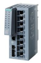
SCALANCE XC208G EEC managed Layer 2 IE switch; IEC 62443-4-2 certified; 8x 10/100/1000 Mbps RJ45 ports; 1x console port; diagnostics LED; redundant power supply; with painted printed circuit boards NAMUR NE21-compliant; temp. range -40 °C to +70 °C; mounting: DIN rail/S7 mounting rail/wall; redundancy functions; Office features (RSTP, VLAN,...); PROFINET IO device; Ethernet/IP-compliant; C-plug slot;
