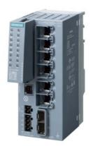
SCALANCE XC206-2SFP EEC managed Layer 2 IE switch IEC 62443-4-2 certified; 6x 10/100 Mbps RJ45 ports; 2x 100/1000 Mbps SFP; 1x console port; diagnostics LED; redundant power supply; with painted printed circuit boards NAMUR NE21-compliant; temp. range -40 °C to +70 °C; mounting: DIN rail/S7 mounting rail/wall; redundancy functions; Office features (RSTP, VLAN,...); PROFINET IO device; Ethernet/IP-compliant; C-plug slot;
