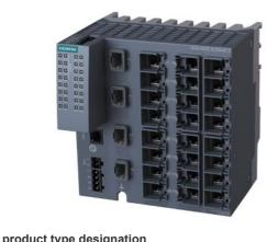
SCALANCE XC224-4C G (E/IP) managed Layer 2 IE switch; IEC 62443-4-2 certified; Full Gigabit; 20x 10/100/1000 Mbps RJ45 ports; 4x 1000 Mbps combo ports (either 1000 Mbps/ SFPs or 10/100/1000 Mbps RJ45 ports can be used); 1x console port; diagnostics LED; redundant power supply; temp. range -40 °C to +70 °C; mounting: DIN rail/S7 mounting rail/wall; redundancy functions; Office features (RSTP, VLAN,...); PROFINET IO device; Ethernet/IP-compliant; C-plug slot; Default EtherNet/IP
