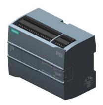
SIMATIC S7-1200F, CPU 1215 FC, compact CPU, DC/DC/relay, 2 PROFINET ports, onboard I/O: 14 DI 24 V DC; 10 DO relay 2 A, 2 AI 0-10 V DC, 2 AO 0-20 mA DC, Power supply: DC 20.4-28.8 V DC, Program/data memory 150 KB
