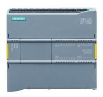
SIPLUS S7-1200 CPU 1214FC DC/DC/DC -25...+55°C with conformal coating based on 6ES7214-1AF40-0XB0 . compact "CPU, DC/DC/DC, ""onboard I/O: 14" "DI 24 V DC;"" ""10 DO 24 V DC; 2" "AI 0-10 V DC, "" Power supply: DC" 20.4-28.8 V DC Program/data memory 125 KB
