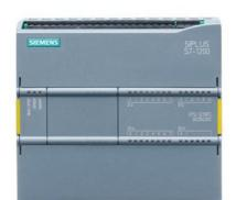
SIPLUS S7-1200 CPU 1214FC DC/DC/relay -25...+55°C with conformal coating based on 6ES7214-1HF40-0XB0 . compact "CPU, DC/DC/relay, ""onboard I/O:" "14 DI 24 V DC;"" ""10 DO relay 2" "A;"" 2 AI 0-10 V DC, Power" supply: DC 20.4-28.8 V DC Program/data memory 125 KB
