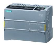
SIPLUS S7-1200 CPU 1215FC DC/DC/DC -25°C...55°C with conformal coating based on 6ES7215-1AF40-0XB0 . compact CPU, DC/DC/DC, 2 PROFINET PORT, "ONBOARD I/O: 14 DI 24VDC; 10 DO" "24V DC 0.5A; 2 AI 0-10V DC, 2" AO 0-20MA DC, POWER SUPPLY: DC 20.4 - 28.8 V DC, PROGRAM/DATA MEMORY 150 KB
