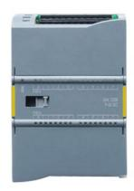
SIPLUS S7-1200 SM 1226 F-DI 16x24 V DC -25...+55°C with conformal coating based on 6ES7226-6BA32-0XB0 F-DI 16X 24 V DC, PROFIsafe, 70 mm overall width, up to PL E (ISO 13849-1)/ SIL3 (IEC 61508)
