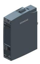
SIMATIC ET 200SP, Digital output module, DQ 8x 24V DC/0,5A Sink Basic, Sink output (NPN, M-switching), Packing unit: 1 piece, fits to BU-type A0, Colour Code CC01, substitute value output, module diagnostics for: supply voltage
