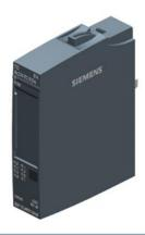
SIMATIC ET 200SP, Digital output module, DQ 8x 24V DC/0,5A Basic, Source output (PNP,P-switching) Packing unit: 10 pieces, fits to BU-type A0, Colour Code CC02, aubstitute value output, module diagnostics for: supply voltage
