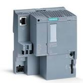
SIMATIC DP, CPU 1510SP-1 PN for ET 200SP, Central processing unit with Work memory 100 KB for program and 750 KB for data, 1st interface: PROFINET IRT with 3-port switch, 72 ns bit performance, SIMATIC Memory Card required, BusAdapter required for Port 1 and 2
