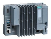
SIMATIC ET 200SP Open Controller, CPU 1515SP PC2, 8 GB RAM, 128 GB CFast with Windows 10 IoT Enterprise 64-bit and S7-1500 Software Controller CPU 1505SP pre-installed, Interfaces: 1x Slot CFast, 1x slot SD/MMC, 1x connection for ET 200SP bus Adapter PROFINET, 1x 10/100/1000 Mbit/s Ethernet, 2x USB 3.0, 2x USB 2.0, 1x display port, Documentation on CFast Restore image on CFast
