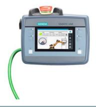
SIMATIC HMI KTP400F Mobile with integrated acknowledgement button, emergency switching-off switch, Touch and Key operation, 4" widescreen TFT display, PROFINET interface, configurable from WinCC Comfort V13 SP1 with HSP
