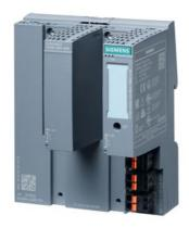
SCALANCE XF204-2BA DNA managed IE Y-switch, IEC 62443-4-2 certified; 4 x 10/100 Mbps, 2 x BusAdapter interface, error signaling contact, set button, redundant 24 V DC power supply, PROFINET device, extended temperature range -40 °C...+70 °C, conformal coating, with electr. manual on DVD, C-plug optional, supplied without BusAdapter
