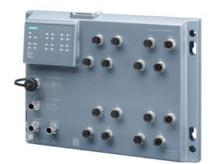
SCALANCE XP216EEC, managed IE switch, with railway approval IEC 62443-4-2 certified; (EN 50155, EN45545); 12x 10/100 Mbps M12 ports, 4x 10/100/1000 Mbps M12 ports IP65, LED diagnostics, error signaling contact, redundant power supply, PROFINET IO device, network management, can be operated in redundant ring, incl. dust caps, incl. electronic manual on CD-ROM, C-plug optional
