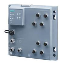
SCALANCE XP208PoE EEC, managed IE switch, 8x 10/100 Mbps IEC 62443-4-2 certified; M12 ports, IP65, LED diagnostics, error signaling contact, redundant power supply, PROFINET IO device, network management, can be operated in redundant ring, dust caps, incl. electronic manual on CD-ROM, C-plug optional
