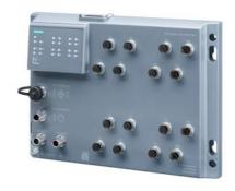
SCALANCE XP216PoE EEC, managed IE switch, with railway approval IEC 62443-4-2 certified; (EN 50155, EN45545); 12x 10/100 Mbps M12 ports, 4x 10/100/1000 Mbps M12 ports IP65, LED diagnostics, error signaling contact, redundant power supply, PROFINET IO device, network management, can be operated in redundant ring, incl. dust caps, incl. electronic manual on CD-ROM, C-plug optional
