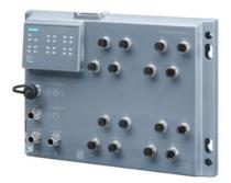
SCALANCE XP216, managed IE switch, 12x 10/100 Mbps IEC 62443-4-2 certified; M12 ports, 4x 10/100/1000 Mbps M12 ports IP65, LED diagnostics, error signaling contact, redundant power supply, PROFINET IO device, network management, can be operated in redundant ring, incl. dust caps, incl. electronic manual on CD-ROM, C-plug optional
