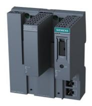
SCALANCE XF204 DNA managed IE Y-switch, IEC 62443-4-2 certified; two BusAdapters BA 2xRJ45 HA preassembled 6DL1193-6AR00-0AA0 4 x 10/100 Mbps, 2 x BusAdapter interface, error signaling contact, set button, redundant 24 V DC power supply, PROFINET device, extended temperature range -40 °C...+70 °C, conformal coating, with electr. manual on DVD, C-plug optional, delivery with BusAdapter
