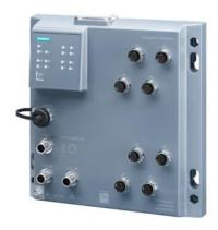
SCALANCE XP208EEC, managed IE switch with railway approval IEC 62443-4-2 certified; (EN 50155, EN 45545); 8x 10/100 Mbps M12 ports, IP65, LED diagnostics, error signaling contact, redundant power supply, PROFINET IO device, network management, can be operated in redundant ring, dust caps, incl. electronic manual on CD-ROM, C-plug optional
