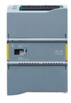
SIPLUS S7-1200 SM 1226 F-DQ 2x relay -25...+55°C with conformal coating based on 6ES7226-6RA32-0XB0 . F-DQ 2x RLY 5A, PROFIsafe, 70 mm overall width, up to PL E (ISO 13849-1)/ SIL3 (IEC 61508)
