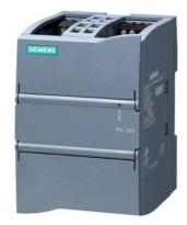
SIMATIC S7-1200 Power Module PM1207 Stabilized power supply input: 120/230 V AC, output: DC 24 V/2,5 A
