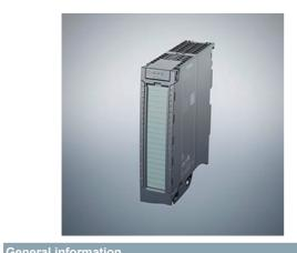
SIMATIC S7-1500, digital output module DQ 16x 230 V AC/2A ST; Relay 16 channels in groups of 2; 4 A per group; switching cycle counter for integrated relay, diagnostics; substitute value: the module supports the safety-oriented shutdown of load groups up to SILCL1 according to EN 62061:2005 + A2:2015, and Category 2 / PL c according to EN ISO 13849-1:2015. front connector (screw terminals or push-in) to be ordered separately
