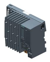
SIMATIC ET 200SP Open Controllers, CPU 1515SP PC F. 4 GB RAM, 30 GB CFAST with WES 7 P 64 bit pre-installed, mit S7-1500 Fail-safe SWC CPU 1505SP F pre-installed Interfaces: 1x slot CFAST, 1x slot SD/MMC, 1x connection for ET 200SP bus adapter PROFINET 1x 10/100/1000 Mbit/s Ethernet, 3x USB, 1x DVI-I graphics card connection, Documentation on DVD, Restore DVD
