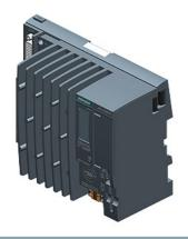
SIMATIC ET 200SP Open Controllers, CPU 1515SP PC F +HMI 512PT, 4 GB RAM, 30 GB CFAST with WES 7 P 64 bit pre-installed, mit S7-1500 Fail-safe SWC CPU 1505SP F pre-installed with WinCC Runtime Advanced V14 pre-installed with 512 PowerTags license, Interfaces: 1x slot CFAST, 1x slot SD/MMC, 1x connection for ET 200SP bus adapter PROFINET 1x 10/100/1000 Mbit/s Ethernet, 3x USB, 1x DVI-I graphics card connection, Documentation on DVD, Restore DVD
