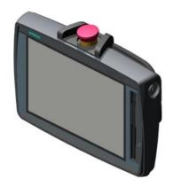
SIMATIC HMI TP1000F MOBILE 10.0" TFT display, 1280x800 pixels, 16 million colors, Touch operation, touch pen, 1x PROFINET/Industrial Ethernet interface, 1x multimedia card, 1x USB, key-operated switch, acknowledgement button, 1 emergency stop/stop button confiigurable from WinCC Comfort V14
