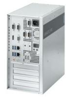
SIMATIC IPC527G (Box PC), Core i7-6700 (4C/8T, 3.4 (4.0) GHz); 512 GB SSD, internal; 8 GB DDR4; Windows 10 Enterprise 2016 LTSB 2x Gigabit Ethernet (IE/PN); 1x DisplayPort, 1x VGA; 4x USB3.0, 2x USB2.0; 2x RS232/485/422 (switchable); 2x RS232, 1x 8bit DIO, 2x PCI; 1x PCIe x16, 1x PCIe x1; 100/240V AC power supply without line cable
