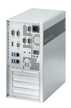
SIMATIC IPC527G (Box PC); Core i5-6500 (4C/4T, 3.2 (3.6) GHz); 1 TB HDD, internal; 8 GB DDR4; without operating system; 2x Gigabit Ethernet (IE/PN); 1x DisplayPort, 1x VGA; 4x USB 3.0, 2x USB 2.0; 2x RS232/485/422 (can be selected); 2x RS232, 1x 8 bit DIO, 2x PCI; 1x PCIe x16, 1x PCIe x1; 100/240 V AC power supply without line cable
