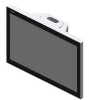
SIMATIC ITC2200 V3 PRO, Industrial Thin Client, 22" widescreen TFT display, capacitive touch sensor, Supported protocols: RDP, VNC, SMARTSERVER, HTML5, etc., standard design, prepared for support arm without expansion elements
