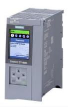
SIMATIC S7-1500F, CPU 1516F-3 PN/DP, central processing unit with work memory 3 MB for program and 7.5 MB for data 1st interface: PROFINET IRT with 2-port switch, 2nd interface: PROFINET RT, 3rd interface: PROFIBUS, 6 ns bit performance, SIMATIC Memory Card required \*\*\*\*approvals and certificates according to entry 109817466 at support.industry.siemens.com to be considered! -
