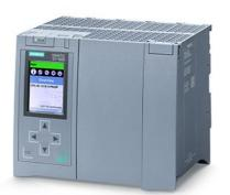
SIMATIC S7-1500, CPU 1518-4 PN/DP, central processing unit with 6 MB work memory for program and 60 MB for data, 1st interface: PROFINET IRT with 2-port switch, 2nd interface: PROFINET RT, 3rd interface: Ethernet, 4th interface: PROFIBUS, 1 ns bit-performance, SIMATIC Memory Card required
