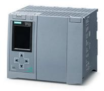
SIMATIC S7-1500F, CPU Bundle consisting of: CPU 1518F-4 PN/DP MFP (6ES7518-4FX00-1AB0), including C/C++ Runtime and OPC UA Runtime license, 9 MB work memory for program and 60 MB for data, 1st interface: PROFINET IRT with 2-port switch, 2nd interface: PROFINET RT, 3rd interface: PROFINET basic services, 4th interface: PROFIBUS, 1 ns bit performance, SIMATIC Memory Card (min. 2 GB) required
