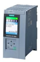
SIMATIC S7-1500F, CPU 1515F-2 PN, central processing unit with work memory 750 KB for program and 3 MB for data, 1st interface: PROFINET IRT with 2-port switch, 2nd interface: PROFINET RT, 30 ns bit performance, SIMATIC Memory Card required
