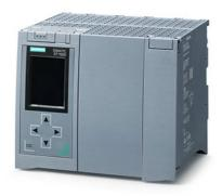
SIMATIC S7-1500F, CPU 1518F-4 PN/DP, central processing unit with 9 MB work memory for program and 60 MB for data, 1st interface: PROFINET IRT with 2-port switch, 2nd interface: PROFINET RT, 3rd interface: PROFINET basic services, 4th interface: PROFIBUS, 1 ns bit-performance, SIMATIC Memory Card required
