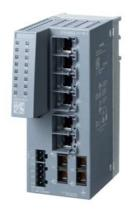
SCALANCE XC106-2, Unmanaged IE switch, 6x 10/100 Mbit/s RJ45 ports, 2x 100 Mbit/s Multimode SC, LED diagnostics, error-signaling contact with set button, redundant Power supply Manual available as a download
