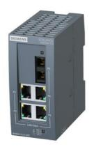
SCALANCE XB004-1G unmanaged Industrial Ethernet Switch for 10/100/1000 Mbit/s; for setting up small star and line topologies; LED diagnostics, IP20, 24 V DC power supply, with 4x 10/100/1000 Mbit/s RJ45 ports electrical and 1 x 1000 Mbit/s SC port optical (multimode, glass), up to max. 750 m Manual available as a download
