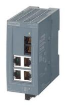
SCALANCE XB004-1LD unmanaged Industrial Ethernet Switch for 10/100 Mbit/s; for setting up small star and line topologies; LED diagnostics, IP20, 24 V AC/DC power supply, with 4x 10/100 Mbit/s twisted pair ports with RJ45 sockets; 1 x 100 Mbit/s single-mode glass FOC port with SC socket; Manual available as a download
