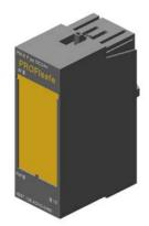
SIMATIC DP, Power Module PM-E F PROFIsafe, f. ET200S; 24 V DC suitable for grounded setup relay for switching the voltage buses P1 and P2 up to Category 3 (EN 954-1)/ SIL2 (IEC61508)/PLD (ISO13849), can also be used in PROFINET configuration with IM 151-3 HF
