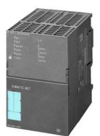
Communications processor CP 343-1 Advanced for connection of SIMATIC S7-300 CPU to Industrial Ethernet: PROFINET IO controller a./o. IO device; RT and IRT, MRP, PROFINET CBA; TCP/IP, ISO, UDP, S7 comm., S5-compat. communication (SEND/RECEIVE) with Fetch/Write RFC1006, Multicast Diagnostic extension, SNMP, DHCP, FTP client/server, e-mail, Gigabit-SS1X RJ45 (10/100/1000) PROFINET interface 2x RJ45 (10/100 Mbit); PROFINET CBA; security (firewall/VPN); PROFInergy
