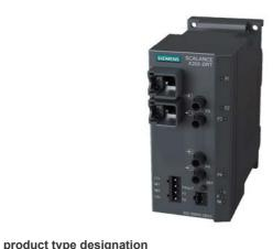
SCALANCE X202-2IRT managed IE IRT switch, 2x 10/100 Mbit/s RJ45 ports, 2x 100 Mbit/s Multimode BFOC, Error signaling contact with set button, Redundant power supply, PROFINET IO device, network management, Redundancy Manager integrated, incl. electron. manual on CD-ROM, C-plug optional
