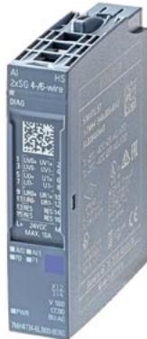
SIMATIC ET 200SP, ANALOG INPUT MODULE, AI 2 X SG 4-/6-WIRE HIGH SPEED, FITS TO BU-TYPE A0, COLOR CODE CC00, CHANNEL DIAGNOSIS, 28/16BIT, +/-0,05%, FOR STRAIN GAUGE FULL BRIDGES
